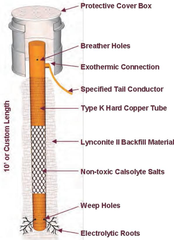
As moisture accumulates, it drips down through the electrode absorbing the salt ions to become a conductive electrolytic solution. This electrolytic solution weeps out of the holes at the bottom of the electrode forming electrolytic roots in the soil.
